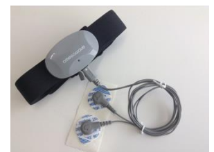
FIGURE 5. Omegawave Bluetooth sensor, strap and electrodes.
