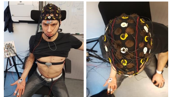
FIGURE 3. 10-20 EEG setup via Mitsar-EEG 202 amplifier and vertex-thenar DC setup via Omegawave.
